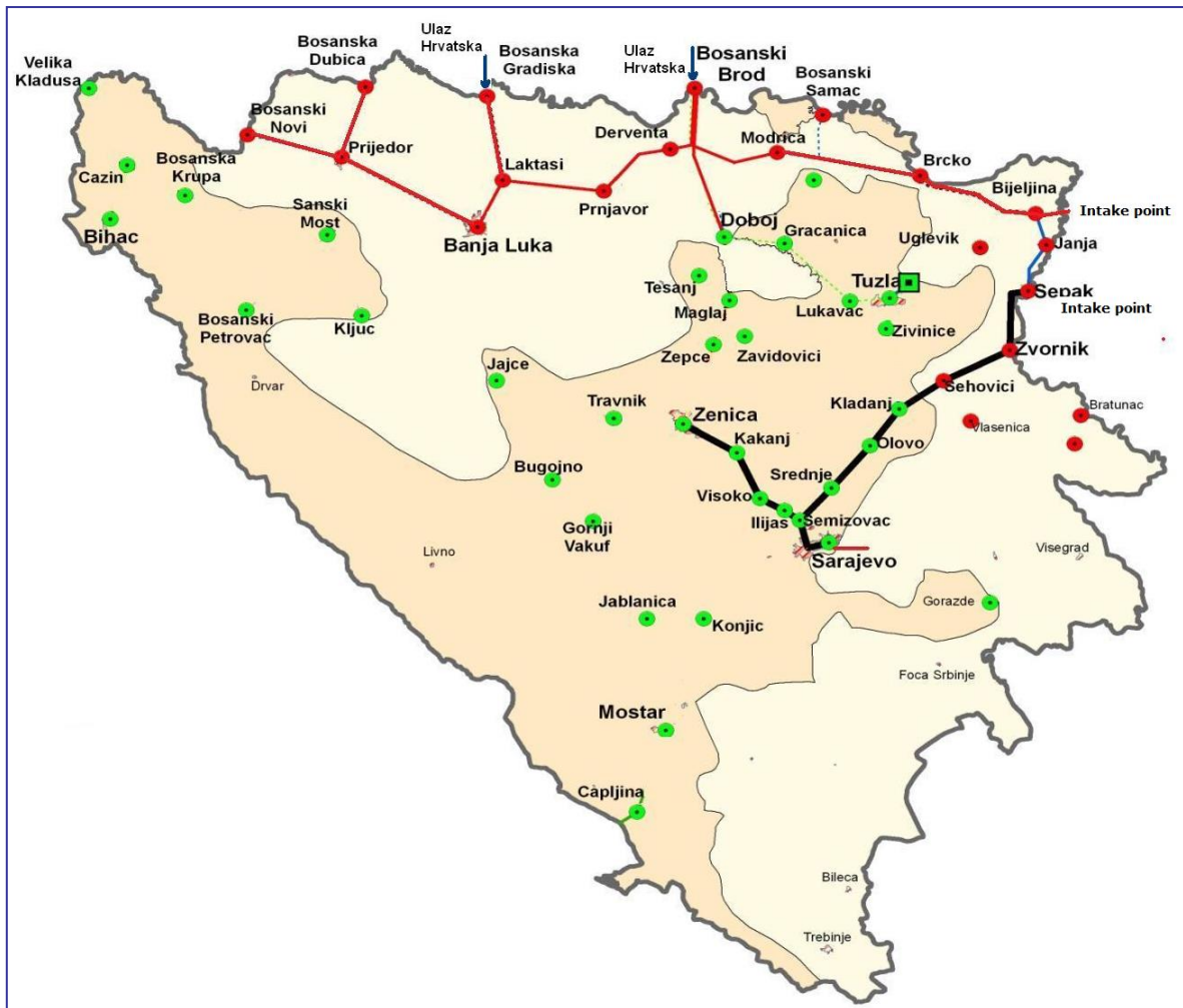
Figure 8: New East Interconnection Gas Transmission Pipeline
